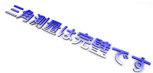
Figure 10. A screenshot of the proposed solution used in a real CAD application, which shows a phrase in Japanese language rendered as a 3D text model, generated by using extrusion from a triangulated mesh.
