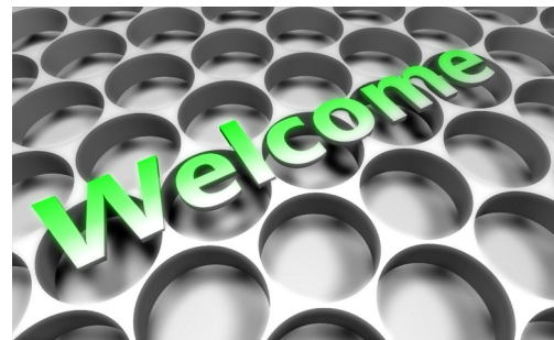
Figure 9. A screenshot of the proposed solution used in a real CAD application, which includes a rectangle with many circular holes as well as 3D text extruded from a triangulated mesh.
